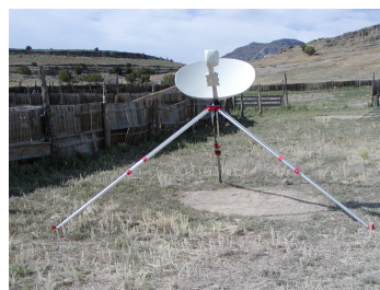
Very wide footprints don't require ballast. Plant the feet well! Legs spread this wide will withstand 60 mph winds.
