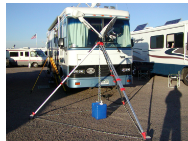
This dish is set 6' high and the legs are spread 7' apart. Ballast is 6 gallons of water (49.8 lbs). Legs are chained together so they won't slip on the hard surface.
