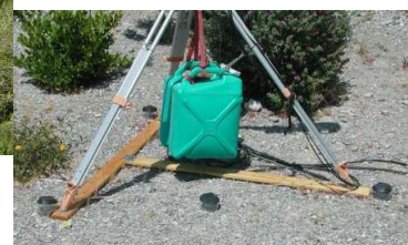
Folding "T" frame is drilled to keep legs from spreading on hard surfaces. It also keeps tripod from sinking in very soft surfaces like sand. Solar charged marker lights make the legs visible at night.
